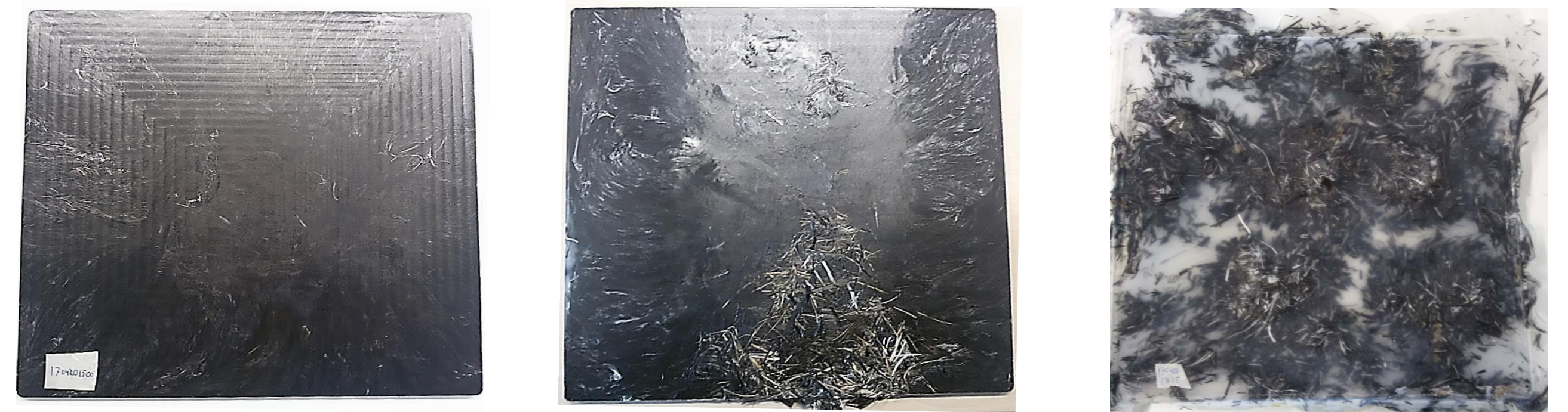
Figure 2: Plates produced at 10% Vf (left) and 20% Vf (middle) by the mixing process with rotating bars and with the non-mixed process (right).
