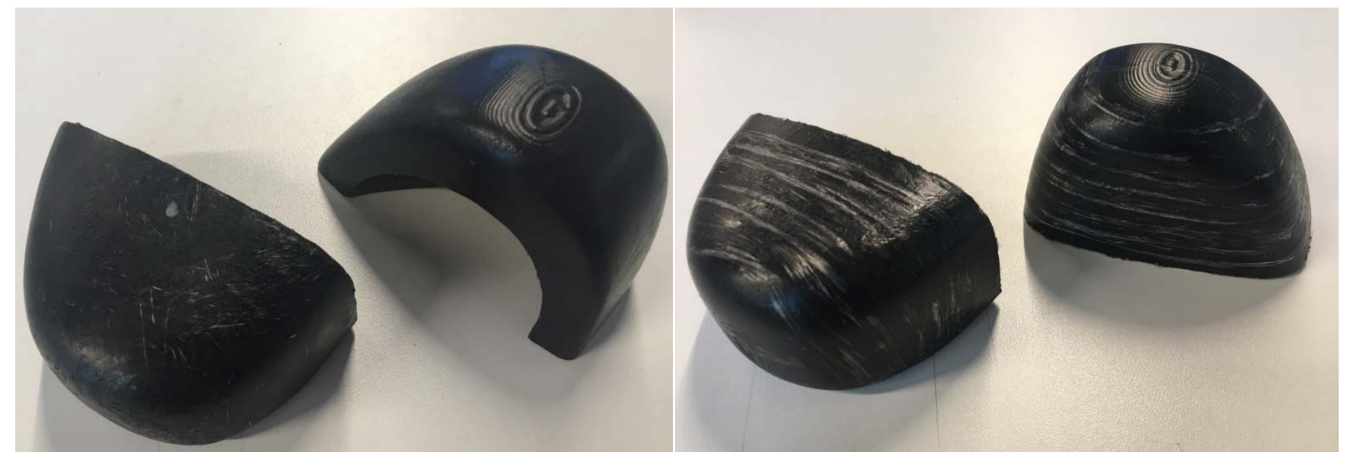
Figure 2: Produced safety shoe noses ( left: W_f 40%, right: W_f 40% + insert)
