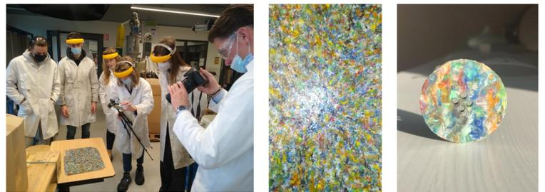
Buttons laser-cut from polyolefin plates while retaining its colours.
