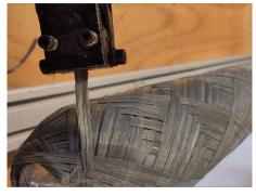
cooling rate, and applied pressure. Perfect consolidation is not always required; for example, minor voids may not affect the performance of a filament-wound pressure vessel.
